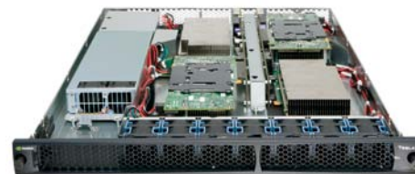
Tesla S2050 GPU Computing System is a 1U system powered by 4 Tesla GPUs and connects to a CPU server.
